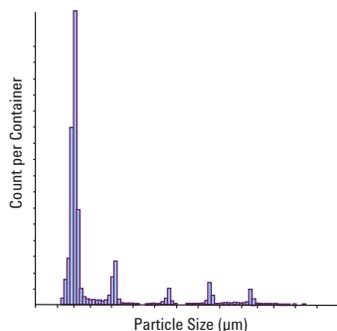
The 7080 AccuSizer, with its ability to count and size individual particles, is a sensitive tool for constructing a material's true particle size. Here, five latex standards of varying size were used in a single sample; all were successfully located by Agilent's 7080 AccuSizer.
