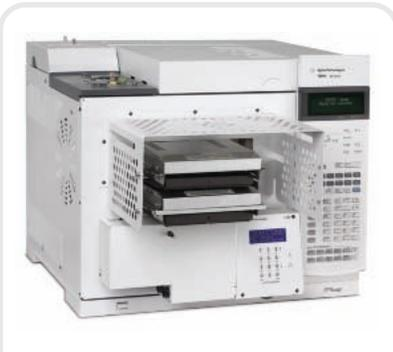
The Agilent LTM System consists of a replacement door for either the Agilent 7890 or the Agilent 6890 that has built-in electronics and slots for inserting from 1 to 4 GC column modules. Programming can be done via Agilent ChemStation software or using a simple keypad control user interface. Up to 10 methods may be stored.
